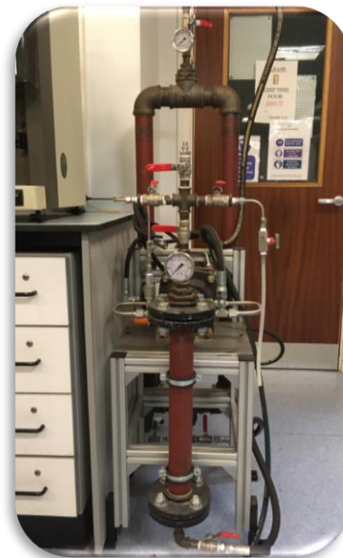
Figure 2. Single-bed PSA unit developed and built at the University of Sheffield for CO 2 separation from gas mixtures.
