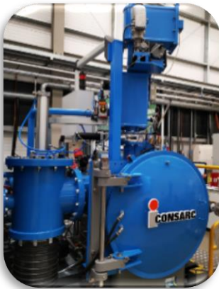
Figure 8a. Left - Vacuum induction melting (VIM) furnace for melting/casting steel in lab, and 8b. Right - an ingot casted from VIM melting.
