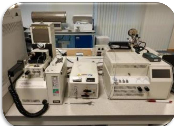
Figure 5a. Left - cutting mill for sample preparation and 5b. Right - pyrolyser
