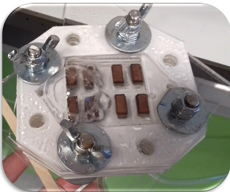
Figure 3. Porous copper monolith electrodes developed and tested as gas diffusion electrodes for carbon dioxide conversion to hydrocarbon in Swansea University
