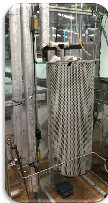
Figure 4. Reactor for the thermochemical conversion of CO 2 to added-value products developed at the University of Sheffield.
