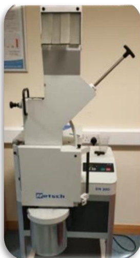
Figure 5a. Left - cutting mill for sample preparation and 5b. Right - pyrolyser
