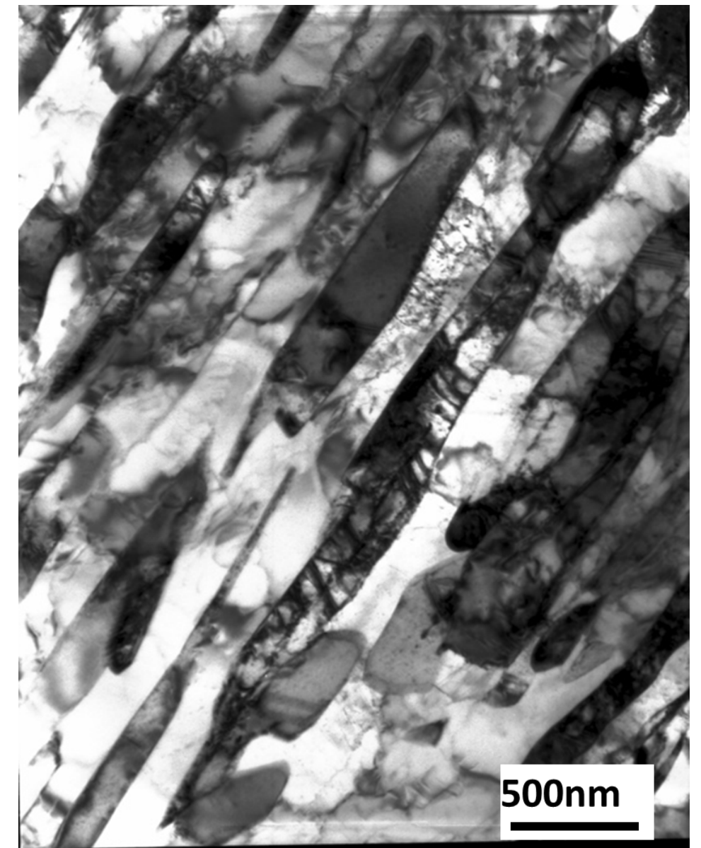
Right: TEM image showing reverted austenite in a tempered martensite matrix in a Super 13Cr steel.
