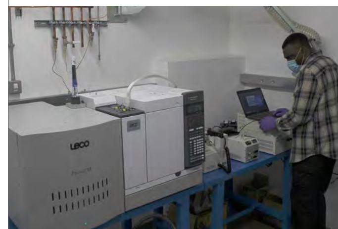
Left: Swansea University PhD researcher Fawaz Ojobowale using the ultra-fast pyrolysis gas chromatography–mass spectrometer (GC-MS)
