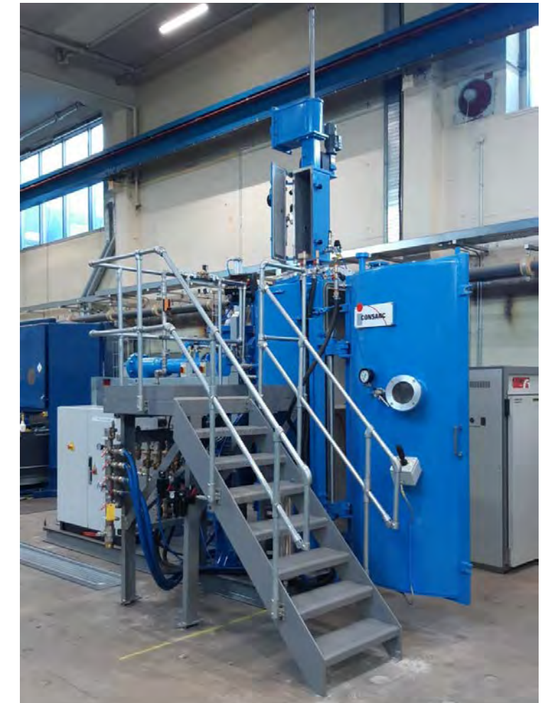
Above: Vacuum induction melt (VIM) for alloy development up to 50kg
