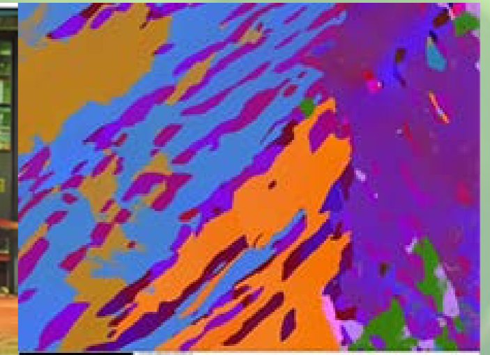
Task 9: Microstructure of Super13Cr steel containing 28% austenite, Euler contrast showing orientation
