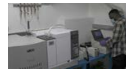
Below: Swansea University PhD researcher Fawaz Ojobowale using the ultra-fast pyrolysis gas chromatography-mass spectrometer (GC-MS)
