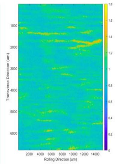
Micro-XRF image of an ingot cast and rolled to 90 mm bar stock 20MnCr5 grade steel showing Mn segregation. The spatial distribution (bands) of Mn is linked to interdendritic segregation during casting (and subsequent rolling deformation for the example shown) with the magnitude and spacing being affected by the cooling rate during (secondary dendrite arm spacing) and subsequent (back diffusion) to solidification.
