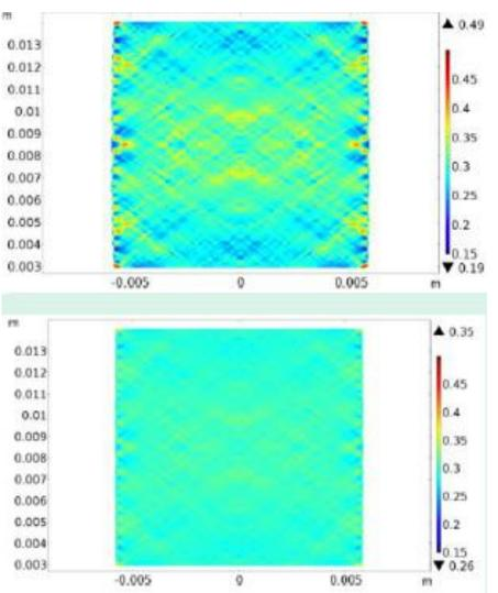
Predicted strain distributions on uniaxial compression for a segregated composition sample (top) and a homogenised sample (bottom) showing the strain inhomogeneity that can arise due to the variation in local strength (from solid solution strengthening) due to compositional (Mn) inhomogeneity.
